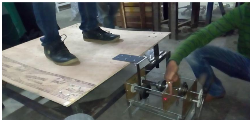
Fig.4 Generation of electricity during downward motion of rack
